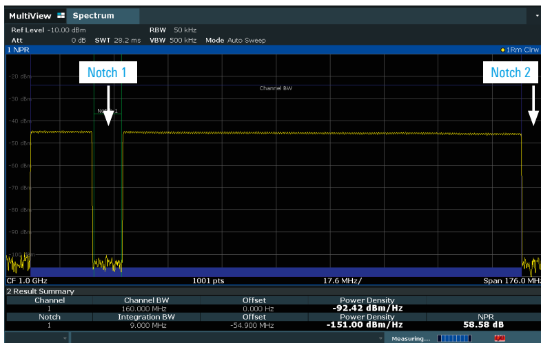
Noise power ratio measurement with the R&S®FSW-K19 option
